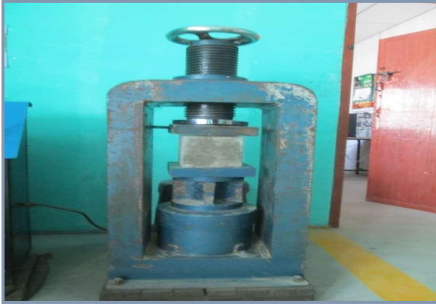
FIG 5.3 CUBE FOR COMPRESSIVE TEST
